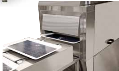
Bretttransportssystemet mater brettene inn i maskinen
